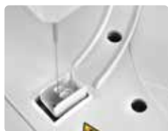
Waterfall probe cleaning
